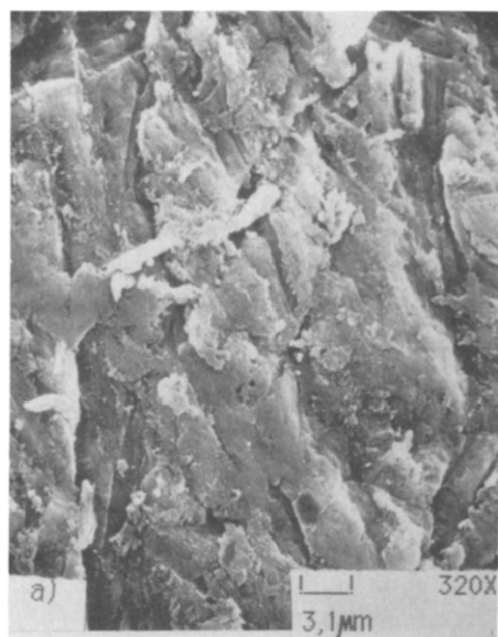
Fig. 2 SEM micrographs of the active layer of the porous gas diffusion electrode on Vulcan XC-72
